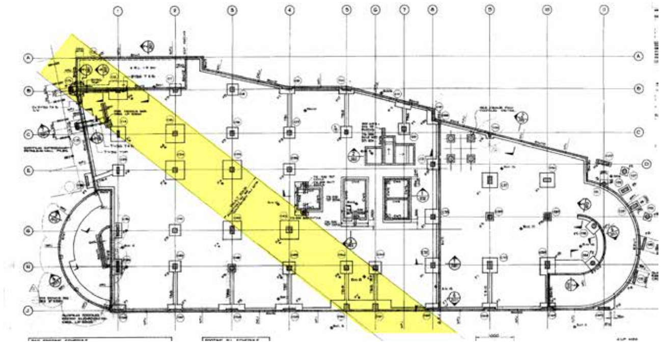
Figure 3: Existing Foundation Plan Showing Fault Zone
